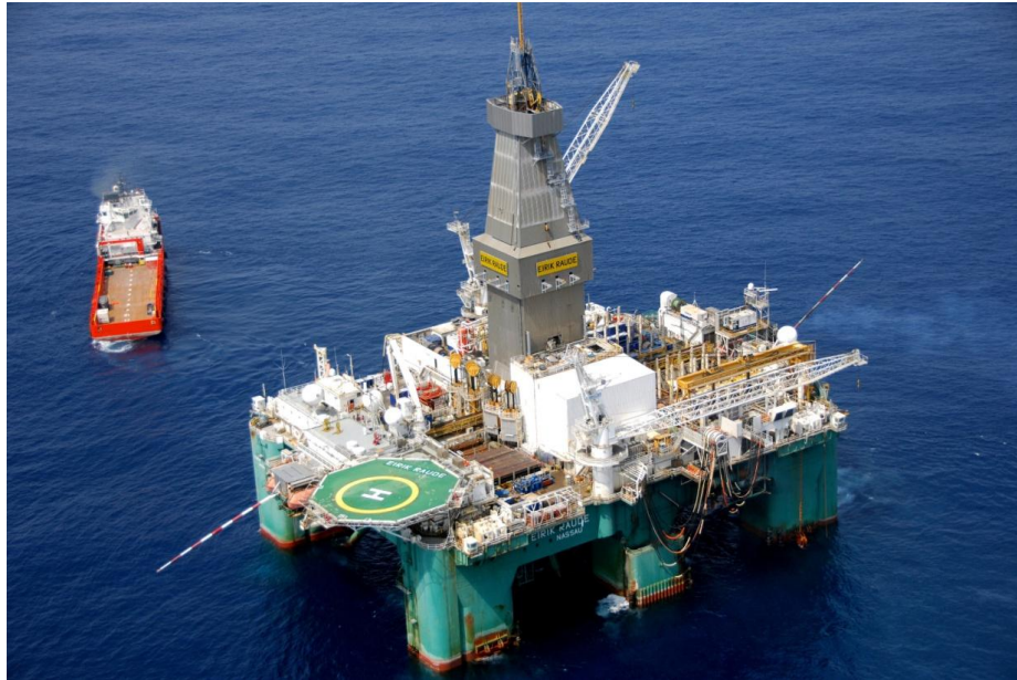
Figure 2.3: 5 th Generation deep water semi-submersible drilling rig 'Eirik Raude' (Ocean Rig, 2014)
